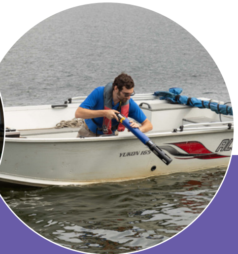
Will Henley, Aquatic Resource Scientist , on Lake Saltonstall in Branford using a state-of-the-art water quality monitoring instrument to measure biological and chemical parameters. Continuous monitoring of lakes plays a crucial role in surface water management. It helps establish baseline data, track trends and identify changes in water quality caused by weather patterns and storm events.
